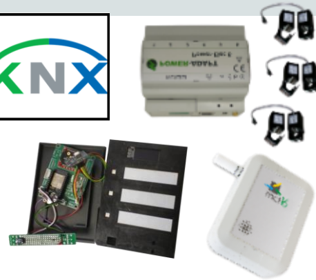
KNX Building Management System + set of heterogeneous IoT devices: different protocols and properties
