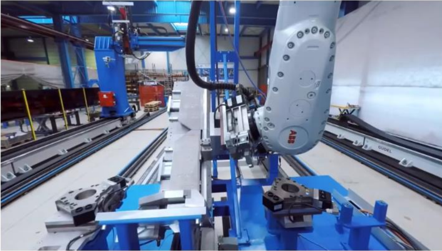
Video 01: Example for state of the art automated steel assembly: ZEMAN's "SBA2 Conti+„ [1]
