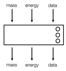
A state defines the internal condition of a planned or abstract system. This includes specific aspects as on, off, open or closed as well as general aspects such as outdoor-air-operation, mixed-air-operation or heating-operation.
