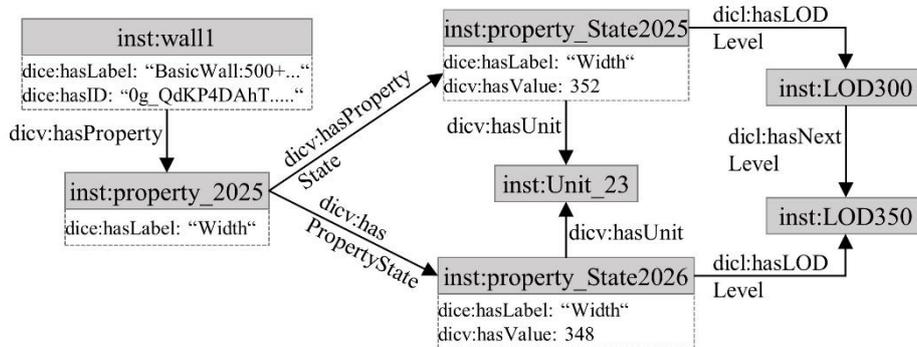
**Fig. 5.** Example BIM data representation at different LOD levels
