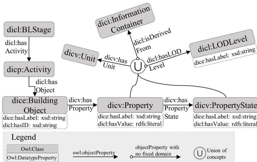
Fig. 4. LOD-sensitive BIM data representation
