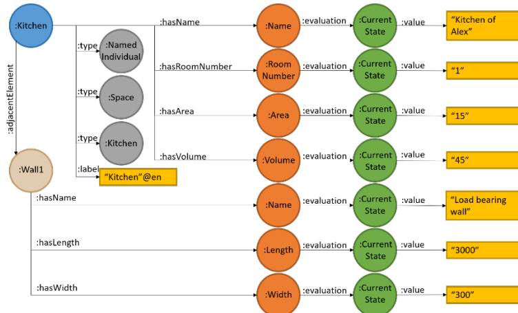
A: RDF graph of a kitchen, based on the open smart home dataset
